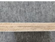
Allply is a tropical hardwood plywood panel that is produced in South America. It has a light-colored tropical hardwood, typically Amescla, veneer on the face and back. The core consists of Amescla combined with Elliotis and Caribbean Pine.
